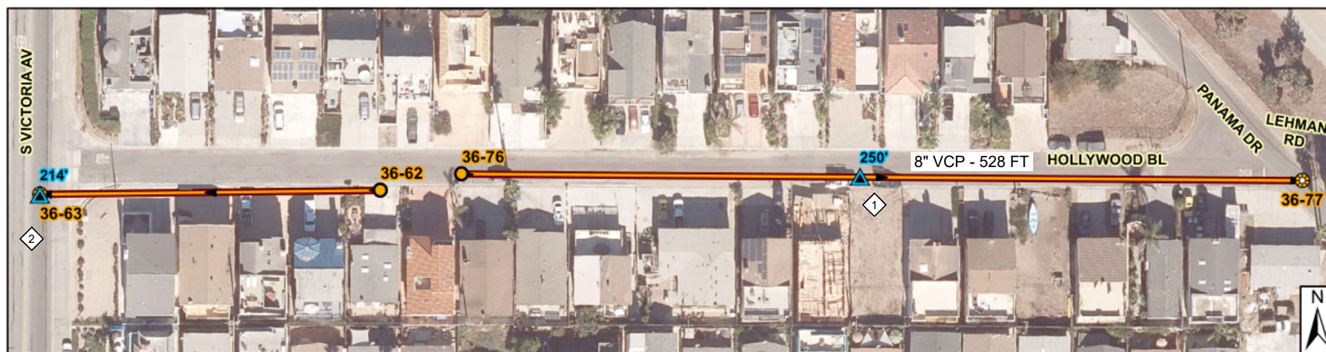
HOLLYWOOD BLVD. (POINT REPAIR) N.T.S.
