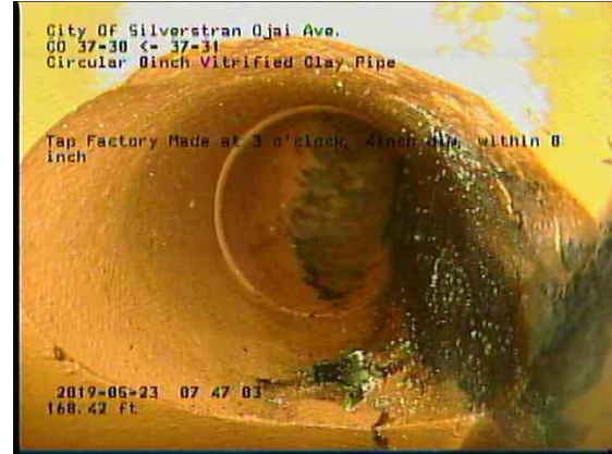
54f29eee-e5a4-4d24-b27f-79483e034471_20190523_074935_805.jpg, 00:09:55, 168.42ft Tap Factory Made at 3 o'clock, 4inch dim, within 8 inch
